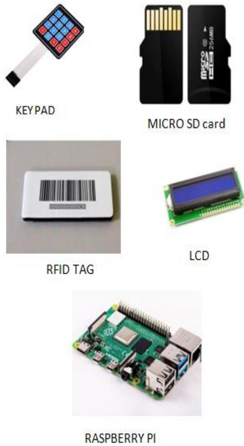
Fig.5 Hardware components of web based Smart Mailbox System
