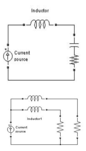
To fix the problem we can add a small resistance in series between voltage source and the capacitors. And we connected a current source in series with an inductor, or a series inductors connected in parallel, and we can add a large resistance in parallel with the inductor and the capacitors.
