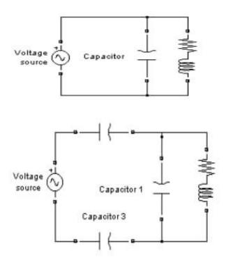
We connected a voltage source in parallel with a capacitor, or a series of capacitor elements in series.
