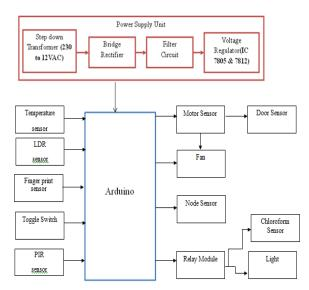
Rectifier is nothing but a Pull-wave rectifier converting Alternating current I/P into a Direct current O/P and then given to the Filter circuit
