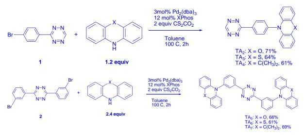
Figure 2: Synthetic route to 3-Monosubstituted Tetrazines (TA2–TA4, Unsymmetrical) and 3,6-Disubstituted Tetrazines (TA5–TA7, Symmetrical) (Qu et al., 2020).
