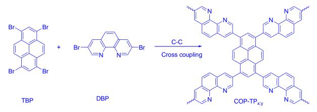
Figure 8: Route of synthesis ogCOP-TP<sub>x:y</sub> by using monomers 3, 6, 8-tetrabromopyrene (TBP) and 3, 8-Dibromo-phenanthroline (DBP)(Y. Liu et al., 2018)
