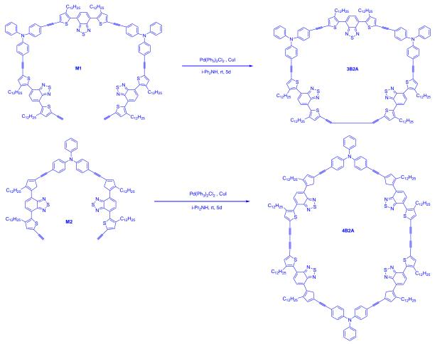
Figure 7:Synthetic route of cyclic conjugated macromolecules 3B2Aand 4B2A. (S. Q. Zhang et al., 2017)
