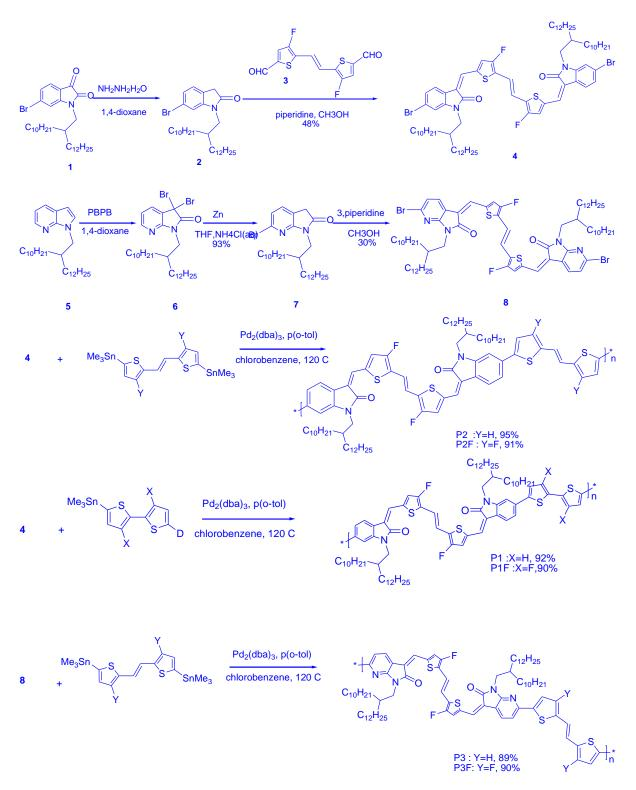
Figure 1: Synthetic route of 4 and 8 monomers and donor-acceptor conjugated Copolymers P1–P3F. (Y. Zhou et al., 2018)
