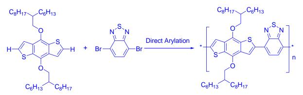
Figure 6: Synthetic Route to the PBDTBT(Polymer benzo[1,2-b:4,5-b']dithiophene 2,1,3-benzothiadiazole)(X. Wang & Wang, 2014)
