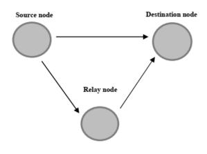
Figure 1: Wireless Cooperative communication using relay node.
