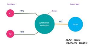
This is a basic perceptron, yet imagine a scenario in which we have numerous inputs and immense data a solitary perceptron isn't sufficient. We should continue expanding the neurons. Also, here is the fundamental neural network having an input layer, hidden layer and output layer.
