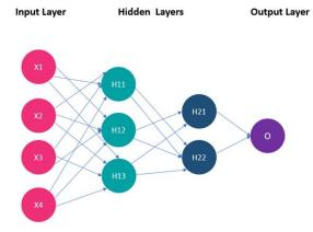
We ought to consistently recall that a neural network has a solitary input layer, output layer however it can have different hidden layers. In the above fig, we can see the example of neural network with one input layer, two hidden layers, and one output layer.
