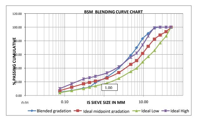
Fig.10 Gradation curve for blended Material curve
