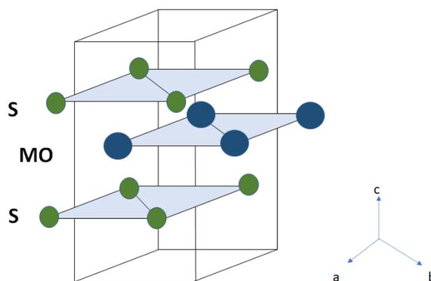
**Fig.1.** Schematic Structure of MoS<sub>2</sub>
