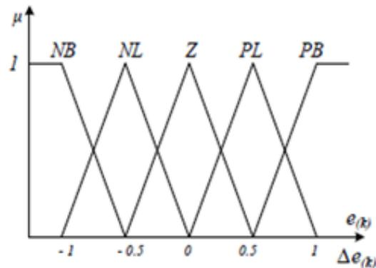
Figure 8. (a) Membership function of FLC for the input variables
