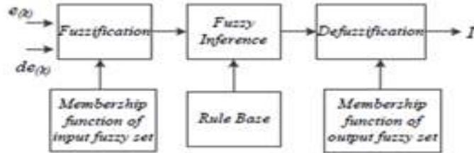
Figure 9. Structure of Fuzzy logic controller
