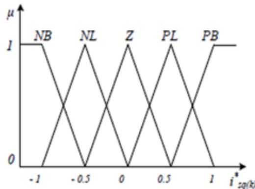
Figure 8. (b) Membership function of FLC for the output variables
