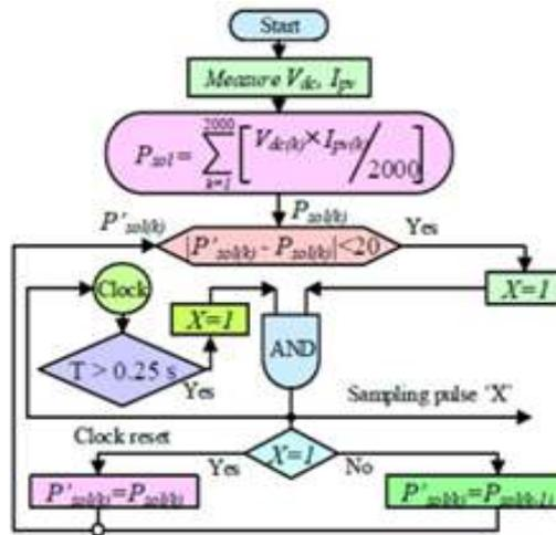
Figure 4. Sampling pulse generation
