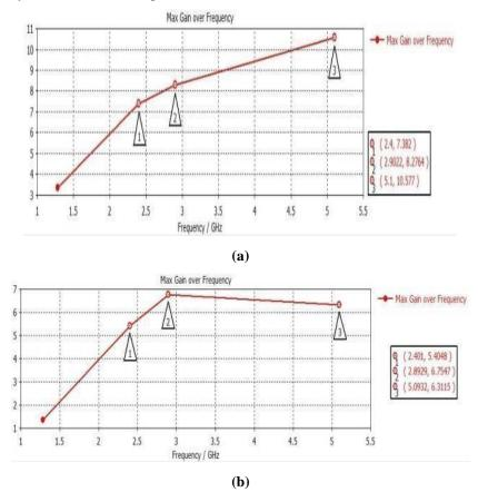
Figure 5. (a) Maximum gain over frequency for RT duroid; (b) Maximum gain over frequency for FR-4
