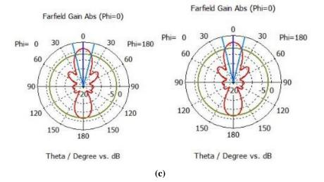
Figure.6 Simulated RDRA array radiation patterns at b) 2.4GHz, c) 2.9GHz, and d) 5.1GHz
