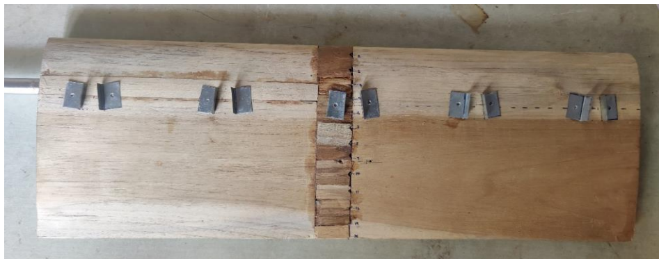
Fig.4 Experimental Model with Pressure tapping and Vortex Generator
