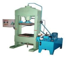
Figure 1. Compression Molding Machine
