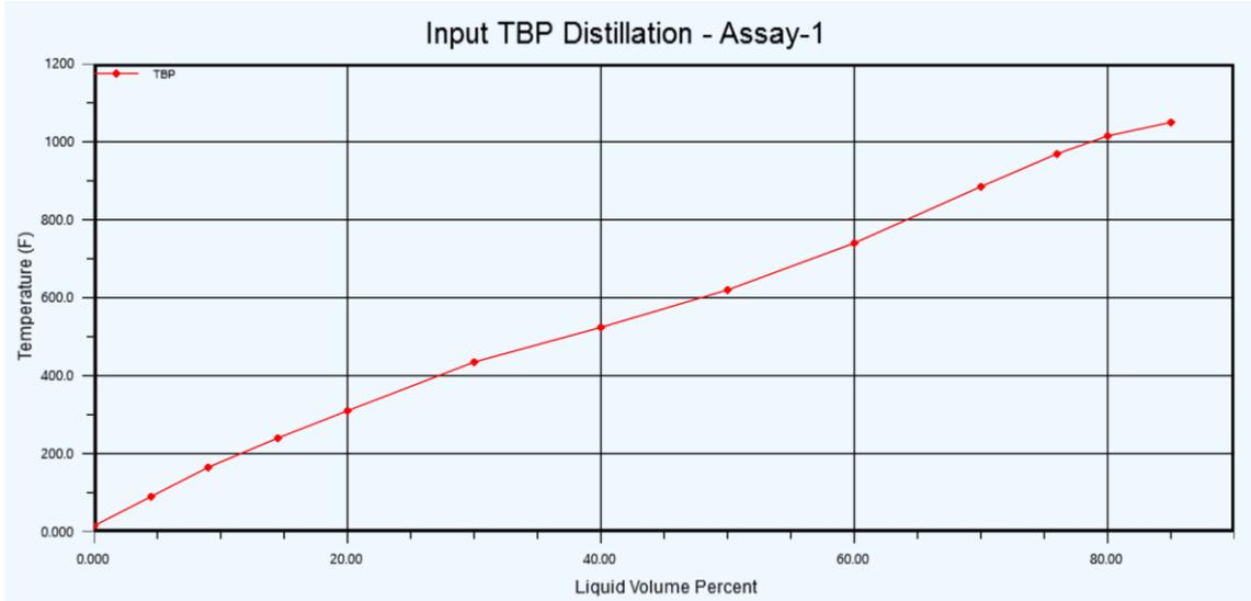
Figure15: TBP plot for input assay
