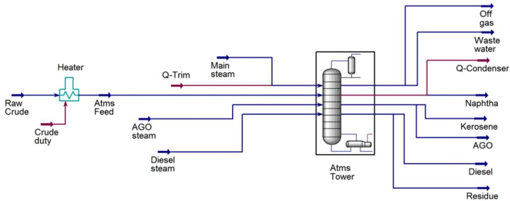
Figure 10: Atmospheric crude distillation flowsheet
