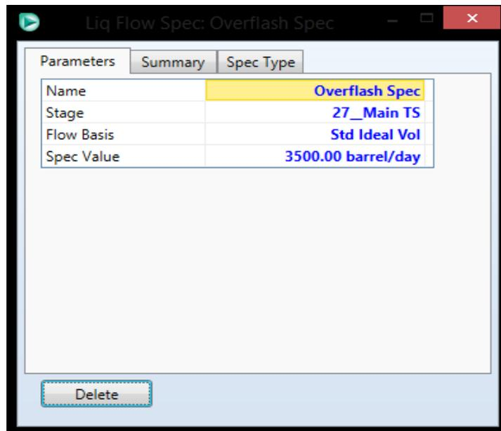
Figure 8: Adding column liquid flow specification
