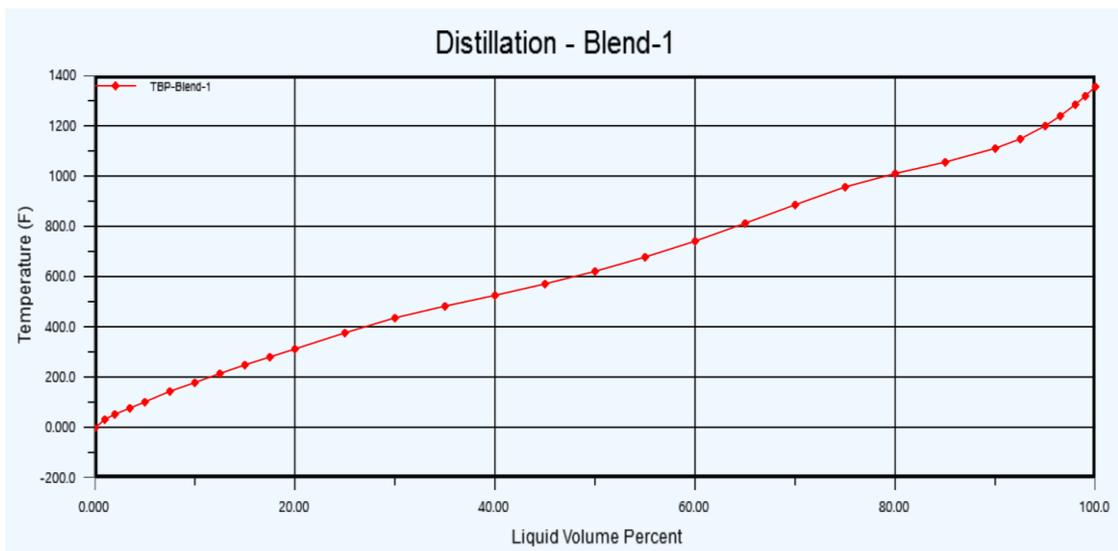
Figure16: TBP plot for output blend
