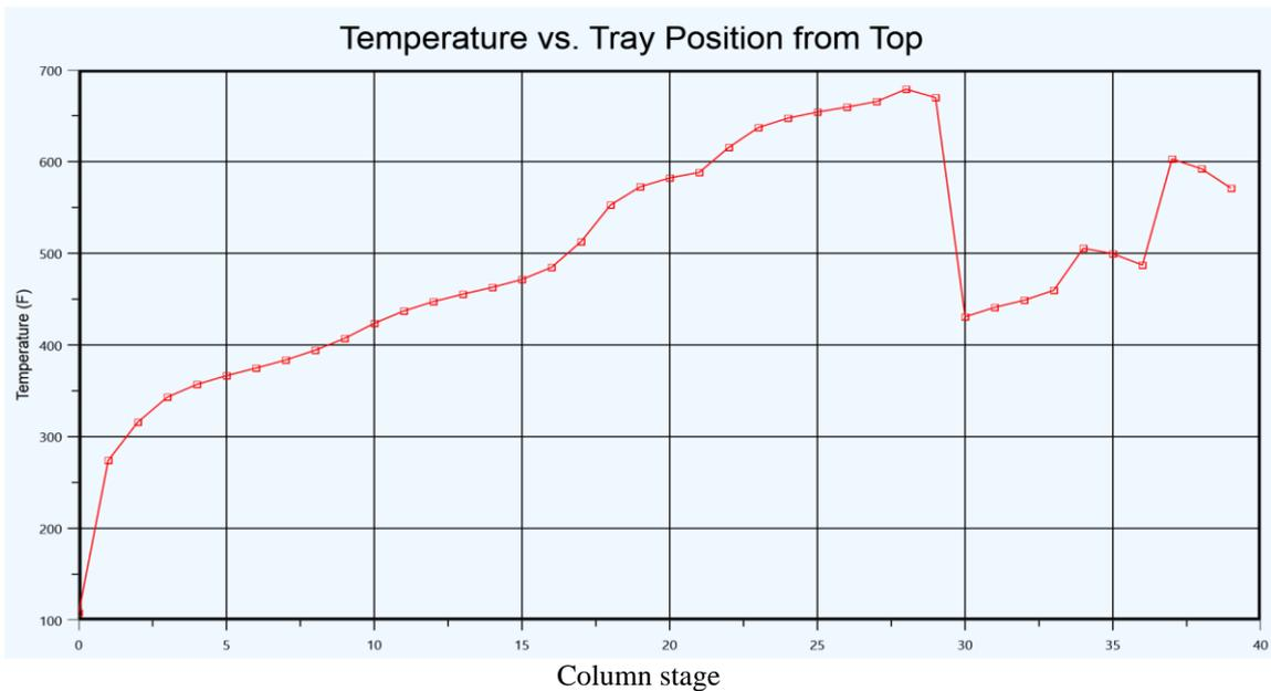
Figure 19: Temperature profile of the crude distillation column
