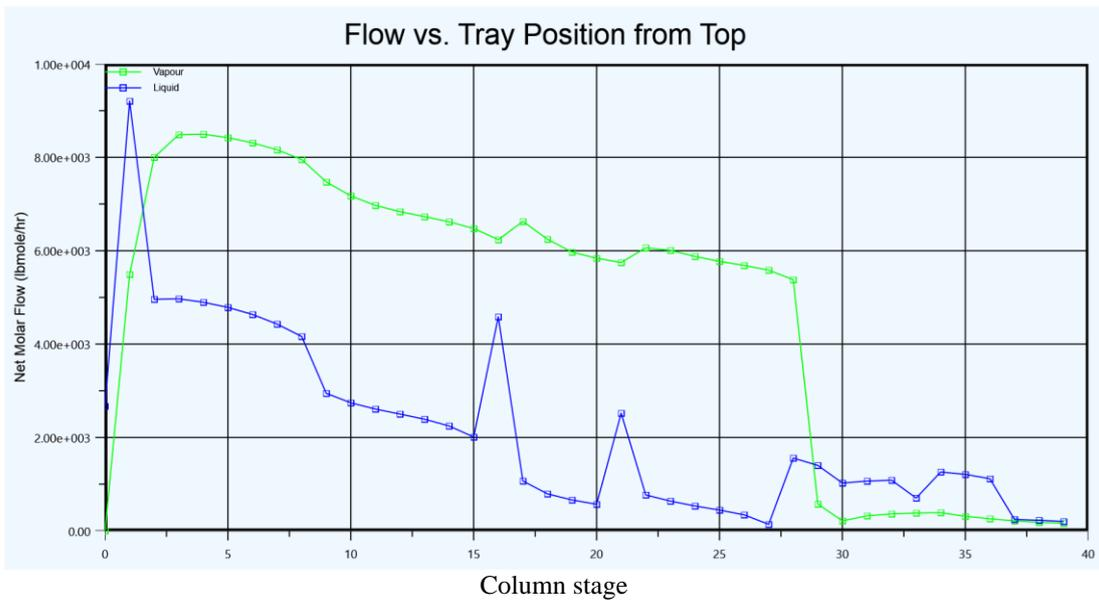
Figure 21: Molar flow profile of the crude distillation column
