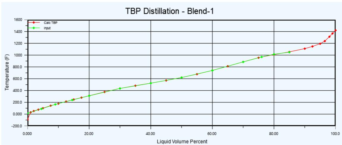
Figure 18: TBP and experimental curve comparison
