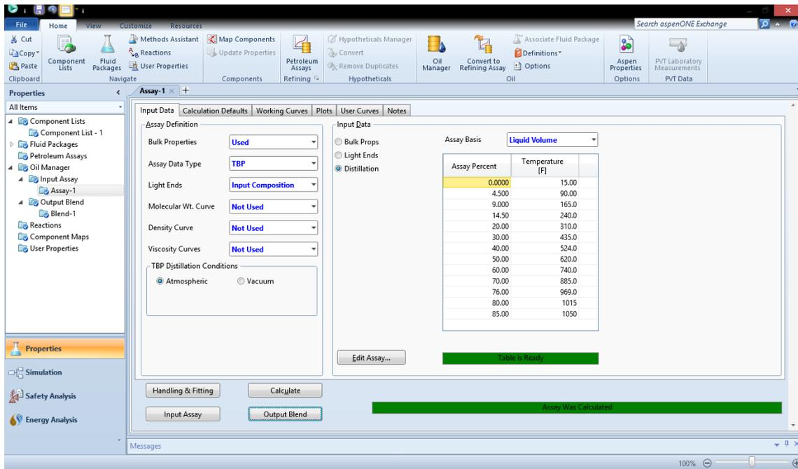
Figure 4: Inputting crude assay distillation parameters
