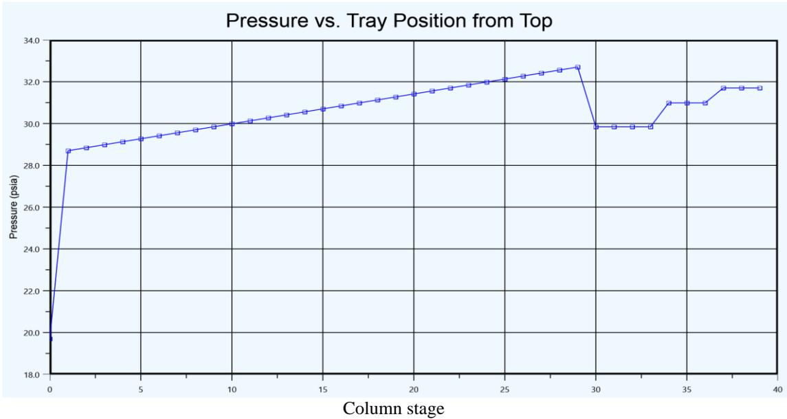
Figure 20: Pressure profile of the crude distillation column
