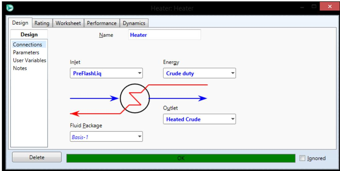
Figure 6: Crude oil heater installed
