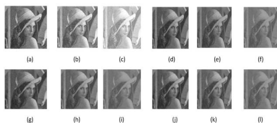
Fig.9. Noisy and restored images: Gaussian noisy images with noise strength (a) SNR=10dB, (b) SNR=5dB, (c) SNR=0dB. Restored images (d) for SNR=10db using NLMF, (e) for SNR=5dB using NLMF, (f) for SNR=0dB using NLMF, (g) for SNR=10dB using NLMF-L, (h) for SNR=5dB using NLMF-L, (i) for SNR=0dB using NLMF-L, (j) for SNR=10dB using NLMF-C, (k) for SNR=5dB using NLMF-C, (l) for SNR=0dB using NLMF-C, filters
