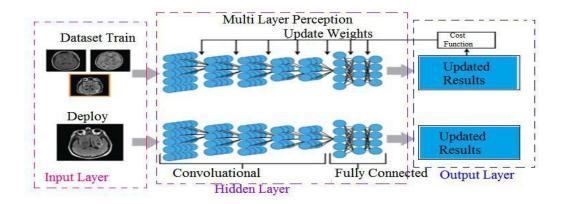
Figure 4. The architecture of the Multi-Layer Perception network
