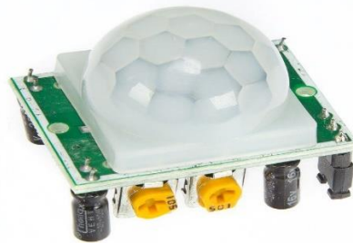
Figure 5 HC-SR501 PIR Sensor
