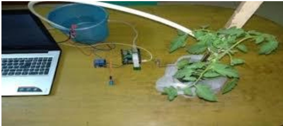
Figure 7 Setup for the proposed scheme, including a tank and leaf detection.
