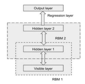
Figure 3.1 Architecture of DBM with 2 RBM
