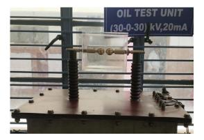
Fig. 2: BDV Test setup
