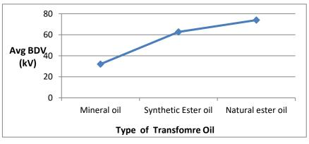
Fig.4 variation of Breakdown voltage in different oils
