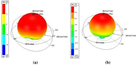
**Figure 5.** Radiation patterns of (a) RHCP antenna (b) LHCP antenna At a resonant frequency  $f_0$ =2.45 GHz
