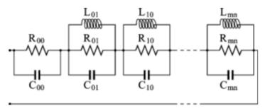
**Figure 12.** Equivalent circuit corresponding to modal expansion of input impedance [5]
