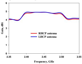
Figure 6 Measured gain plots of the antenna prototypes
