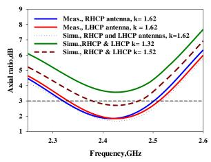
Figure 4. Simulated (parametric) and measured axial ratio plots
