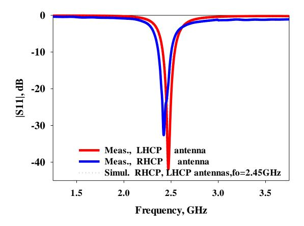
Figure 3. |S11| plots of RHCP and LHCP antennas.
