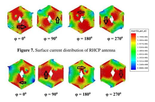
Figure 8. Surface current distribution of LHCP antenna
