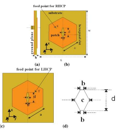
Figure 1. Geometry of the proposed antenna. (a) side view (b) Top view of RHCP antenna (c) Top view of LHCP antenna. (d) central irregular hexagonal slot geometry, Guided wavelength  $\lambda g = 0.0604$  m, a = 17.244mm (0.285  $\lambda g$ ), b=1mm (0.0166  $\lambda g$ ), c = 7mm(0.116 $\lambda g$ ), d = 11.4mm(0.189 $\lambda g$ ), k = 1.62, L = W = 50 mm (0.8278  $\lambda g$ ). X (21mm,19 mm), Y (21mm, 31mm).
