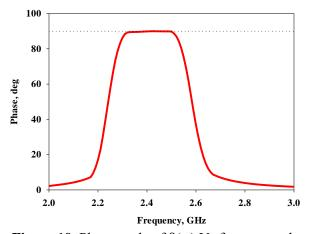
**Figure 19.** Phase angle of  $\beta(\omega)$  Vs frequency plot
