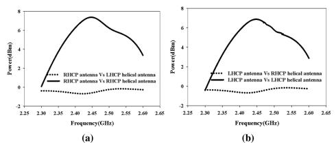
**Figure 9.** Sense of direction of polarisation using helical antennas, when tested (a) RHCP antenna (b) LHCP antenna
