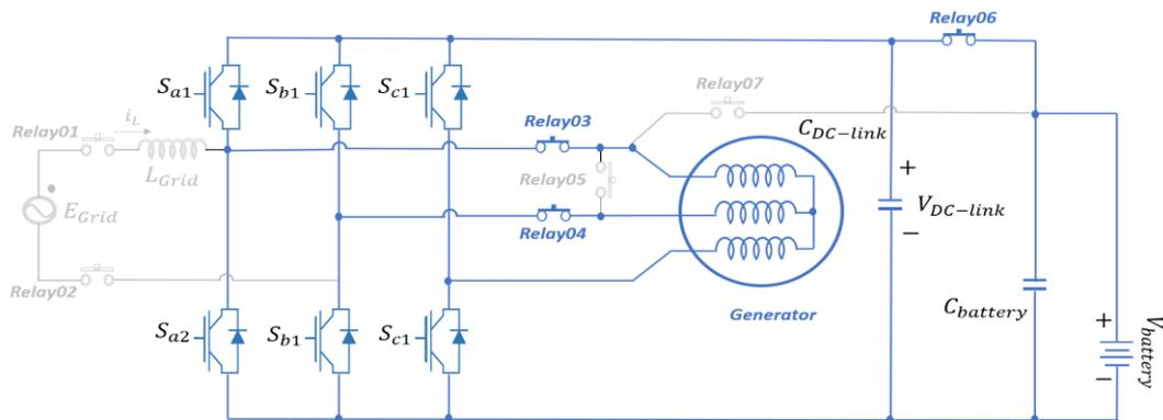
**Fig. 1. (a) starter-generator drive mode**
