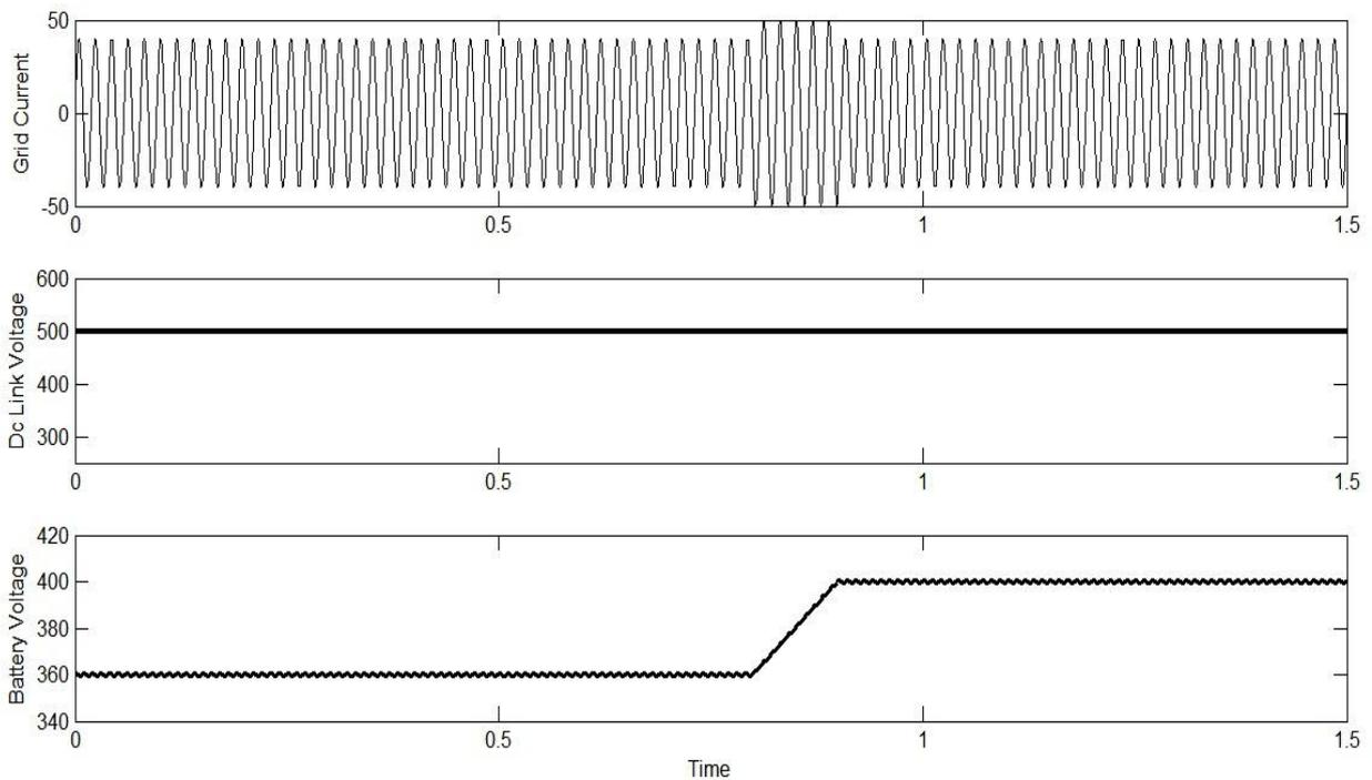
**Fig. 6. (b)** For the Improved integrated charging system, simulation waveforms depict various charging strategies: voltage control, which varies between battery voltage
