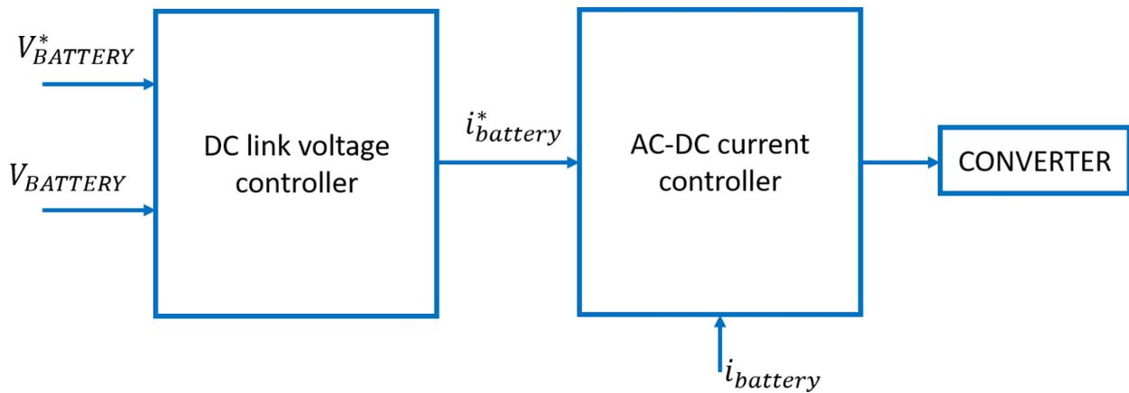
**Fig. 4. DC-DC Converter control system**
