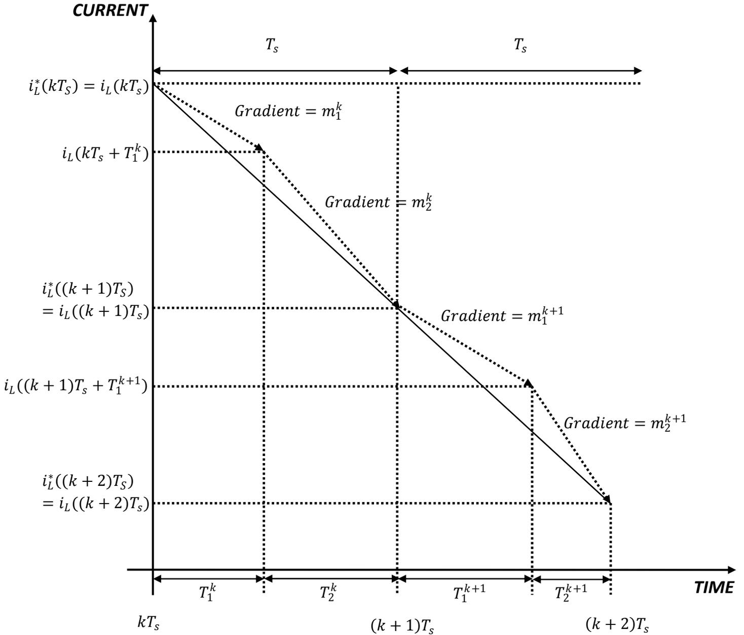
**Fig. 3. The slope of current & time-span in recommended Enhanced MPC technique**
