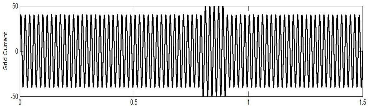
**Fig.5.(a)Controlling the current using the MPCC technique Simulation result**
