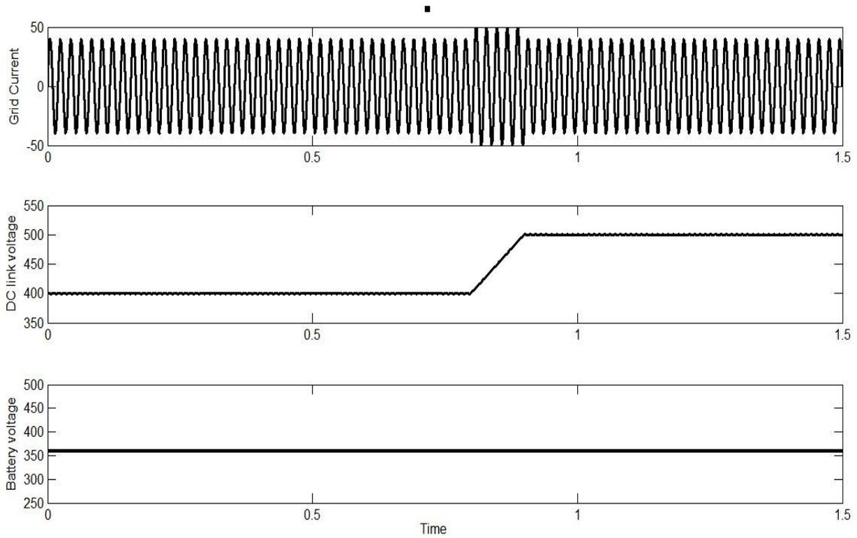
**Fig. 6.(a)** For the Improved integrated charging system, simulation waveforms depict various charging strategies: voltage control, which varies between DC link voltage
