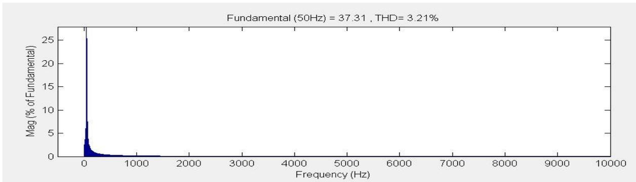
**Fig.7. (a) PI Controller THD waveform**
