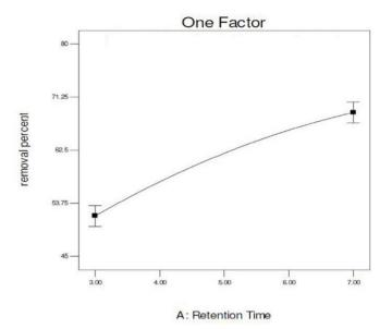
*Fig. 4.* The effect of retention time on the efficiency of dye removal (input dye concentration = 25 mg/l)
