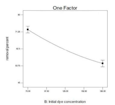
Fig. 5. The effect of initial dye concentration on the dye removal efficiency (retention time = 5 hours)
