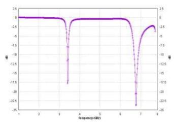
Figure 4: Conventional Antenna reflection coefficient plot in decibel
