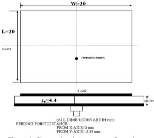
Figure 1: Conventional Antenna configuration
