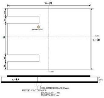
Figure 3: Proposed Antenna (Ground View)
