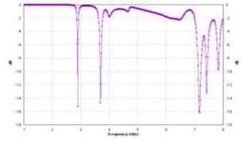
Figure 5: Proposed Antenna reflection coefficient pattern in decibel
