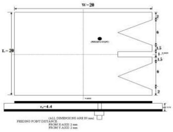
Figure 2: Proposed Antenna (Top View)
