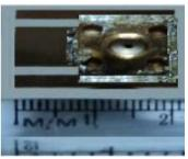
Fig 10(b): Bottom Layer of Proposed Antenna
