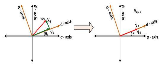
Fig. 1 Phasor representation of grid voltage on two coordinate axis
