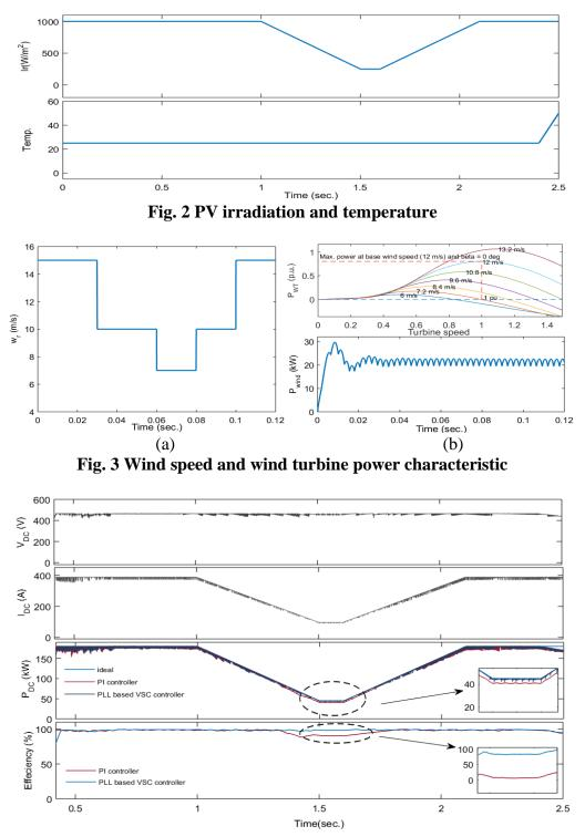
Fig. 4 DC-link voltage, current, and power under the proposed controller
