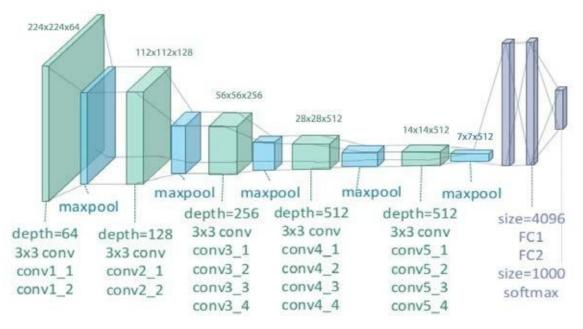
Fig. 5 Block diagram of VGG19
