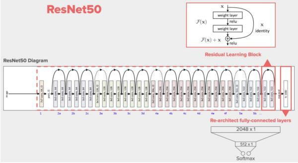
Fig. 3 Architecture of ResNet50
