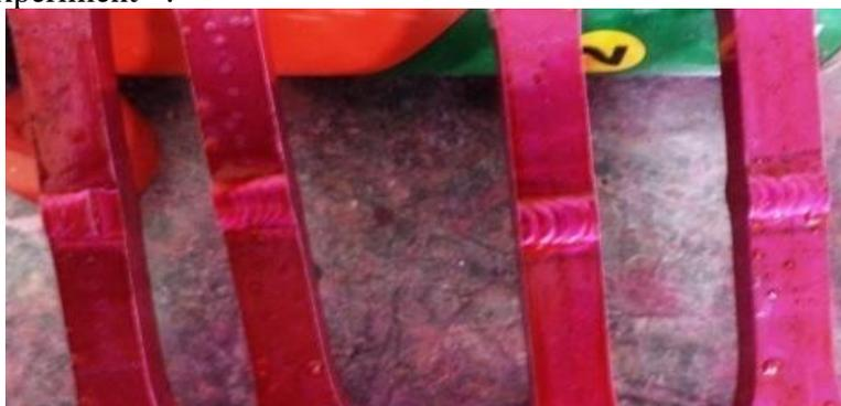
**Fig.2. Samples after putting on penetrant**
