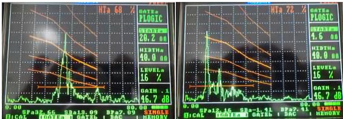
**Fig.8. Increase in signal strength due to an increase in load in defect weldments.**
