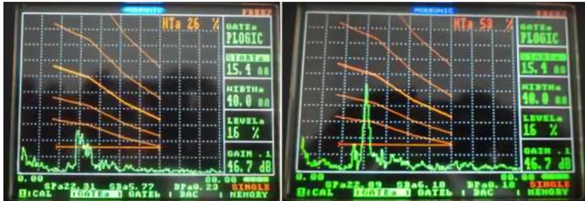
**Fig.7. Increase in signal strength due to an increase in load in good weldment.**
