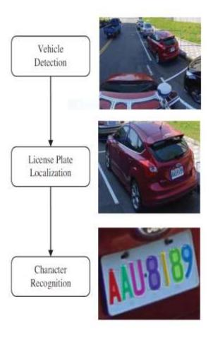
Figure:3Stages of proposed license plate recognition system
