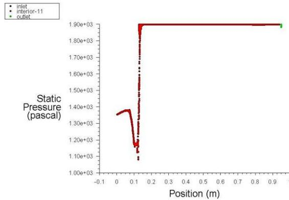
**Figure 15. Variation in backpressure on engine during the flow through EDS – VI at constant Load 5 Kg.**
