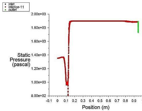
**Figure 12. Variation in backpressure on engine during the flow through EDS – III at constant Load 5 Kg.**
