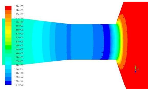
**Figure 8. The pressure contour for EDS – Vat at constant Load 5 Kg.**
