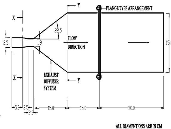
**Figure 17. Schematic view of Exhaust Discharger System (EDS)**
