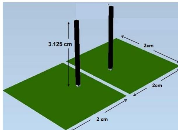
**Figure 1: General representation of proposed antenna**
