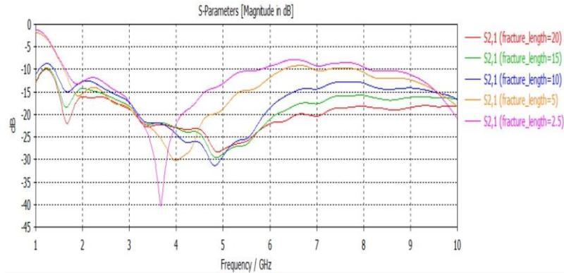
**Figure 5: S21 parameter for the various fracture length**
