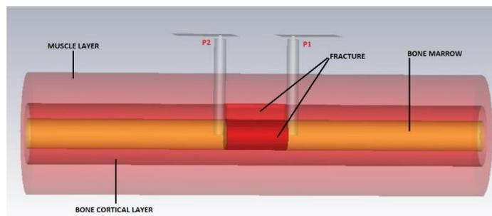
**Figure 3: front view of the phantom with the fracture and antenna**
