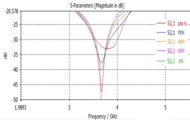
**Figure 4: S21 parameter for various stages of fracture**
