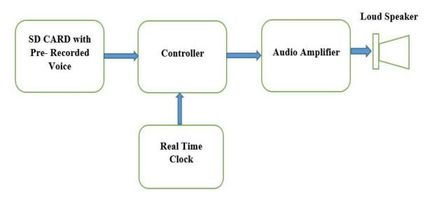
**Fig 4. Block Interconnection of Tablet Reminder**
