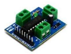
Fig 5. Motor driver IC (L293D)
