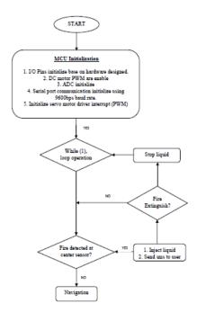
Fig 7. Flow chart for the robot
