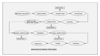
Fig: 13. Flow chart of manufacturing process
