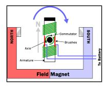
Fig: 7. DC motor arrangement
