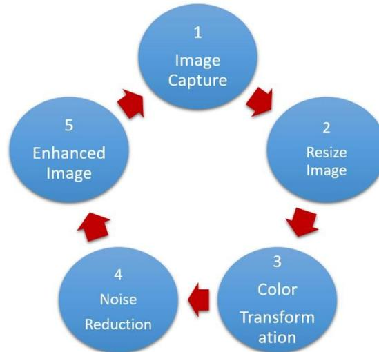
Image Capture, Size Conversion, Color Translation, Noise Removal, and Image Enhancement are all part of the suggested technique. It's all laid out in full in the accompanying diagram (Figure 1)
