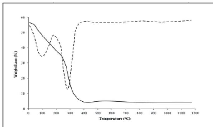
**Fig. 15: Thermogram of mesoporous  $\text{Fe-AlPO}_4$**
