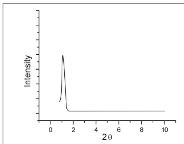
**Fig: 8: Powder XRD spectrum of mesoporous Mg-AlPO<sub>4</sub>**
