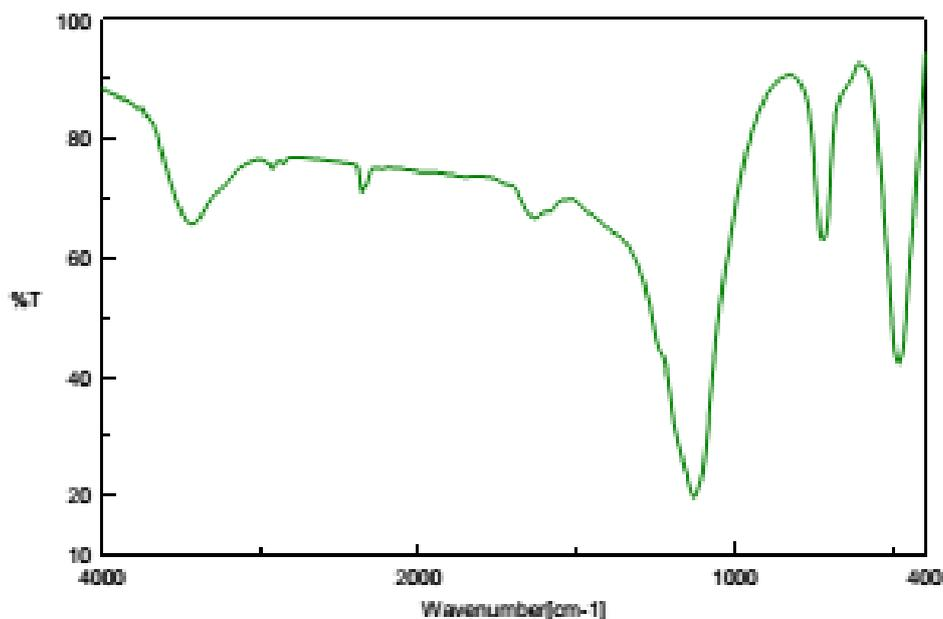
**Fig 1: FT-IR spectrum of mesoporous  $\text{AlPO}_4$**
