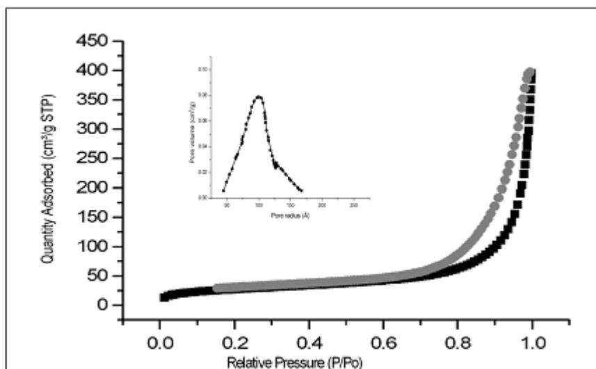
**Fig. 12: N<sub>2</sub> sorption isotherm and pore distribution plot for mesoporous Mg-AlPO<sub>4</sub>**
