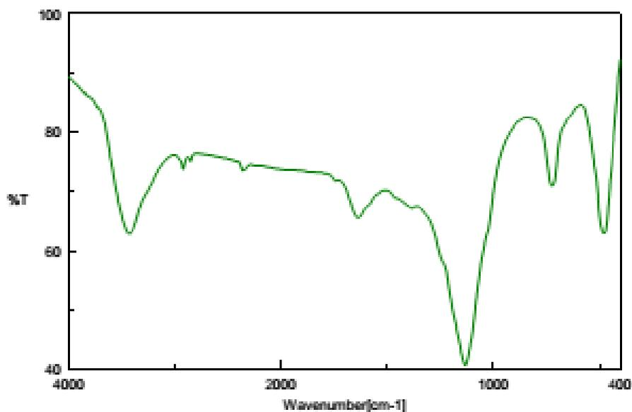
**Fig 2: FT-IR spectrum of mesoporous  $\text{Zn-AlPO}_4$**
