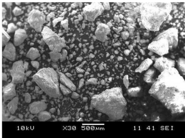
**Figure 19: SEM image of mesoporous Fe-AlPO<sub>4</sub>**
