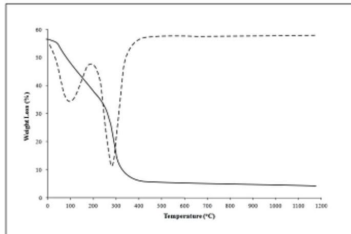
**Fig. 14: Thermogram of mesoporous  $\text{Zn-AlPO}_4$**
