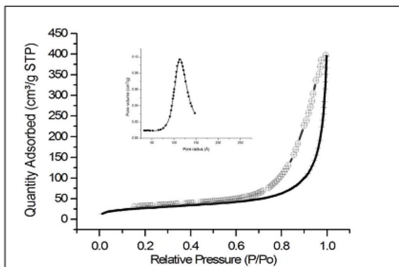
Fig: 10: N<sub>2</sub> sorption isotherm and pore distribution plot for mesoporous Zn-AlPO<sub>4</sub>
