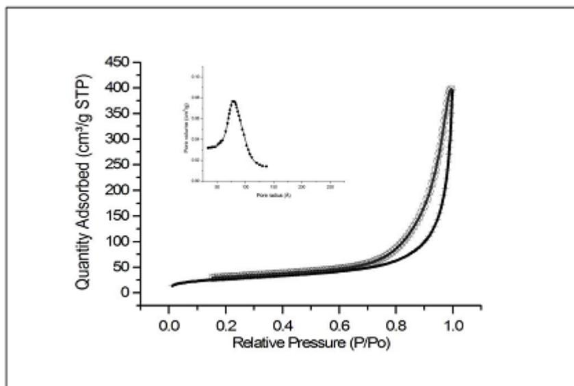
**Fig. 11: N<sub>2</sub> sorption isotherm and pore distribution plot for mesoporous Fe-AlPO<sub>4</sub>**
