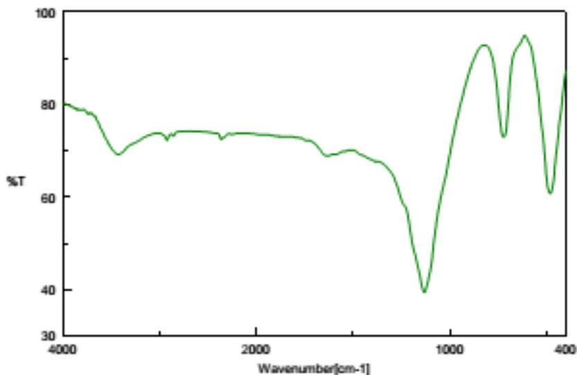
**Fig. 3 : FT-IR spectrum of mesoporous Fe-AlPO<sub>4</sub>**
