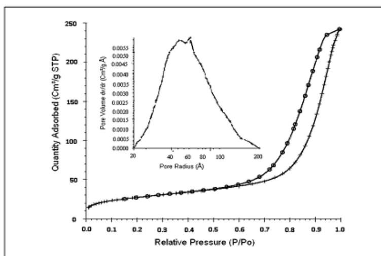
Fig:9: N<sub>2</sub> sorption isotherm and pore distribution plot for mesoporous AlPO<sub>4</sub>
