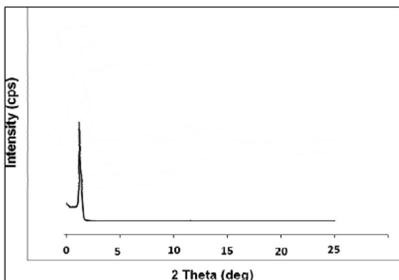
**Fig:6: Powder XRD spectrum of mesoporous Zn-AlPO<sub>4</sub>**
