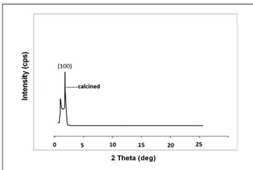
**Fig: 5: Powder XRD spectrum of mesoporous AlPO<sub>4</sub>**
