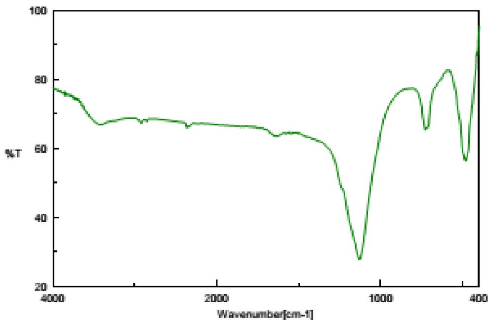
**Fig. 4 : FT-IR spectrum of mesoporous Mg-AlPO<sub>4</sub>**
