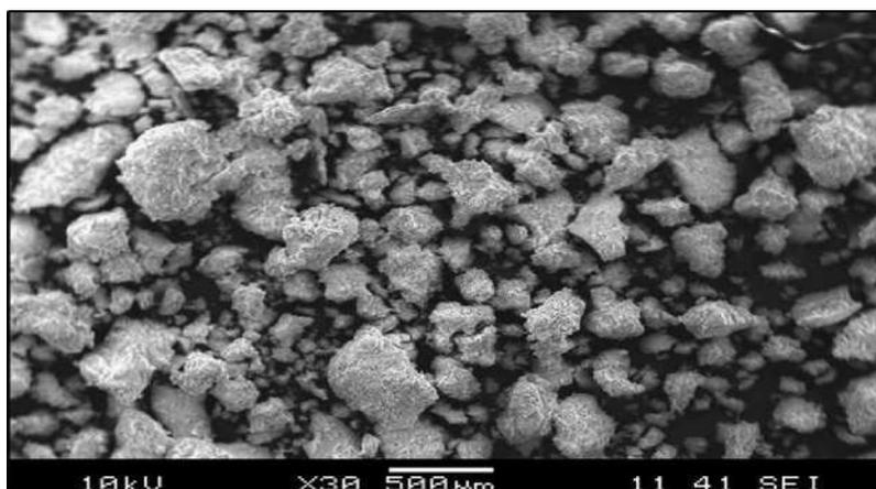
**Figure 17 SEM image of mesoporous AlPO<sub>4</sub>**
