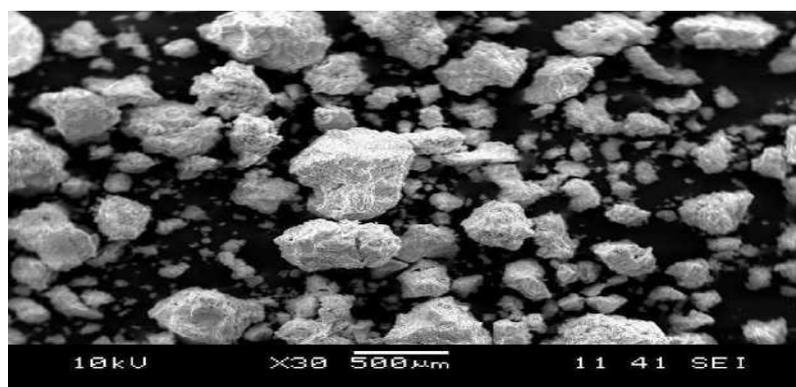
**Figure 18 SEM image of mesoporous Zn-AlPO<sub>4</sub>**
