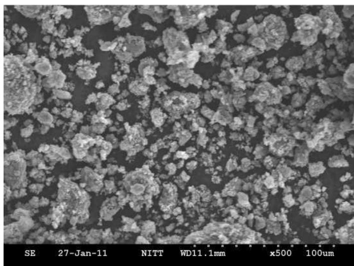
**Figure 20 SEM image of mesoporous Mg-AlPO<sub>4</sub>**
