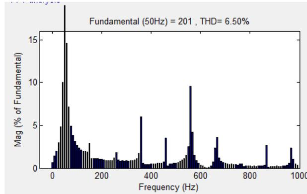
Fig. 13 THD of output voltage
