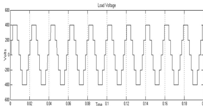
Fig. 11 shows the output voltage with a resistive load ( $R = 10$  and  $L = 5$  mH).
