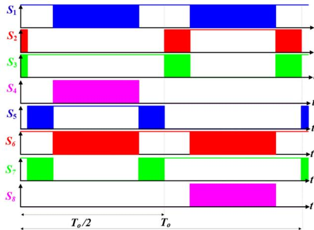
Fig. 7 displays the signals that operate the five-position inverter
