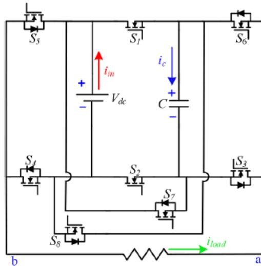
Fig. 2 shows the single-phase configuration of the five-position inverter.
