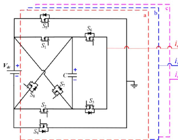
Fig. 1 The main schematic for the suggested five-position inverter is shown.
