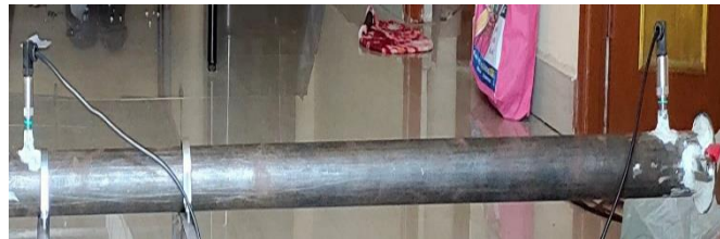
Figure. 4.2 Pressure sensor and its positions at the either end of Driven section
