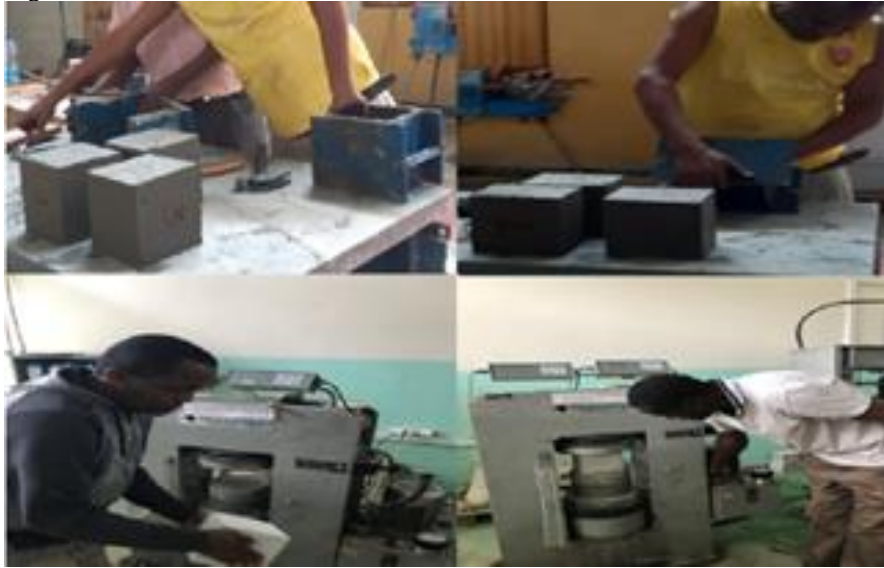
Figure 1.1 Compressive Strength Testing For Cube Samples
