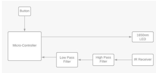
**Fig. 2:** Block diagram of the proposed system
