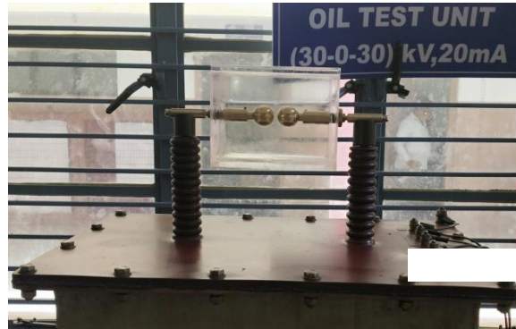
Figure 5: BDV TEST SETUP
