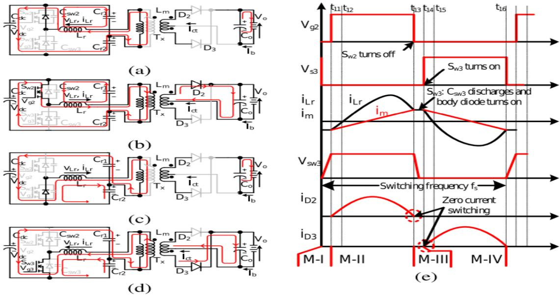
**Fig. 4:** Operating Modes of HBLLC Converter a) Mode 1 b) Mode 2 c) Mode 3 d) Mode 4 e) Switching Waveforms of the HBLLC converter
