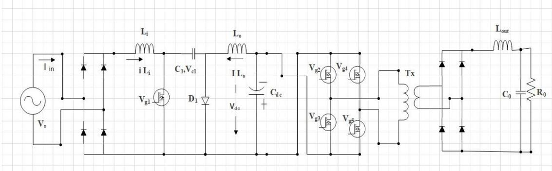
**Fig. 5:** Configuration of CUK Converter fed isolated PSFB
