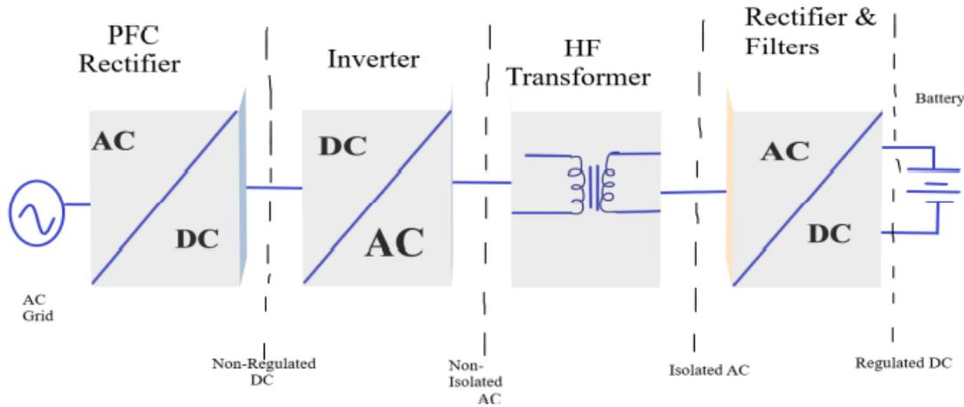
**Fig. 1:** EV Charging Circuit using PFC and HF Transformer
