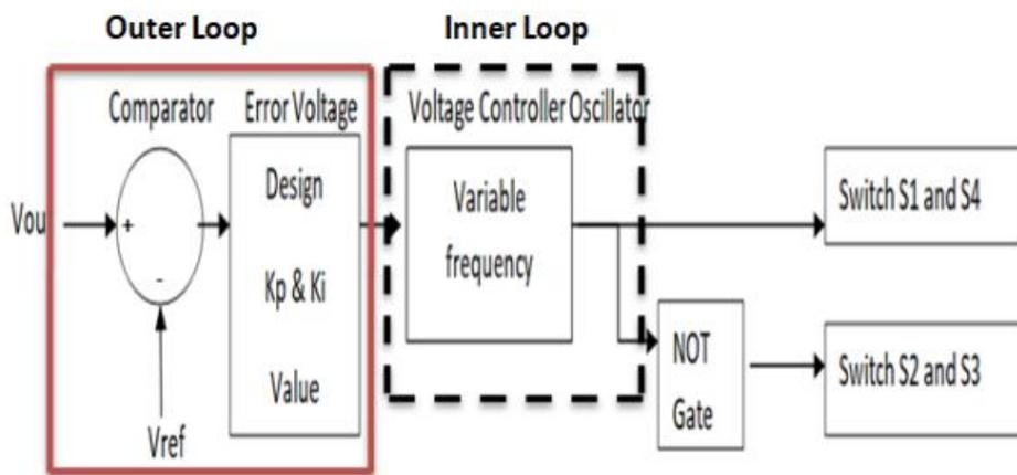
**Fig. 8:** Control loop diagram of HBLLC Converter
