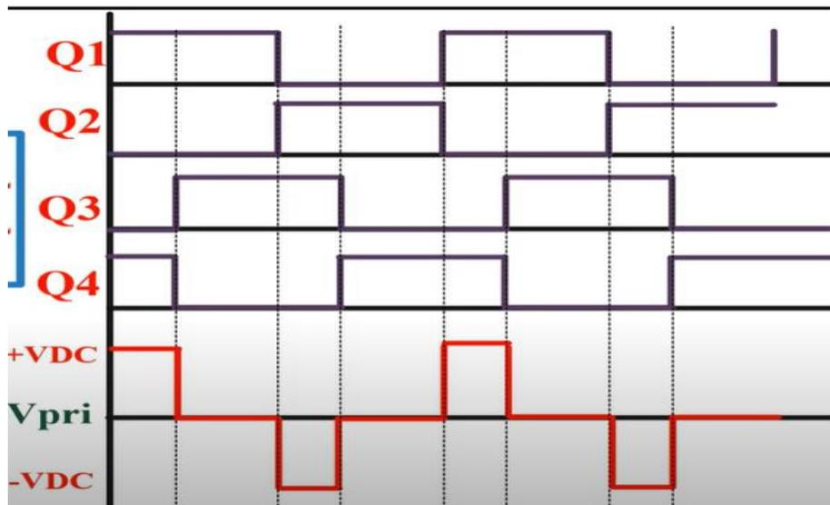
Fig. 6: Switching Waveforms of PSFB converter.
