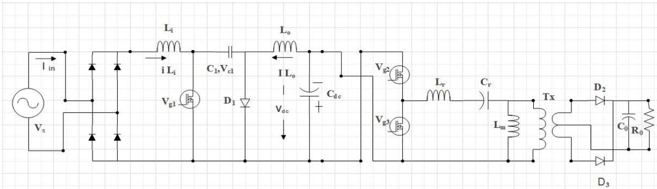
Fig. 2: Configuration of CUK converter fed isolated HLLC
