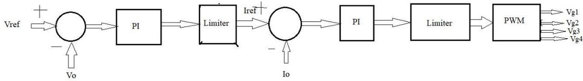
**Fig. 9:** Control loop diagram of PSFB Converter
