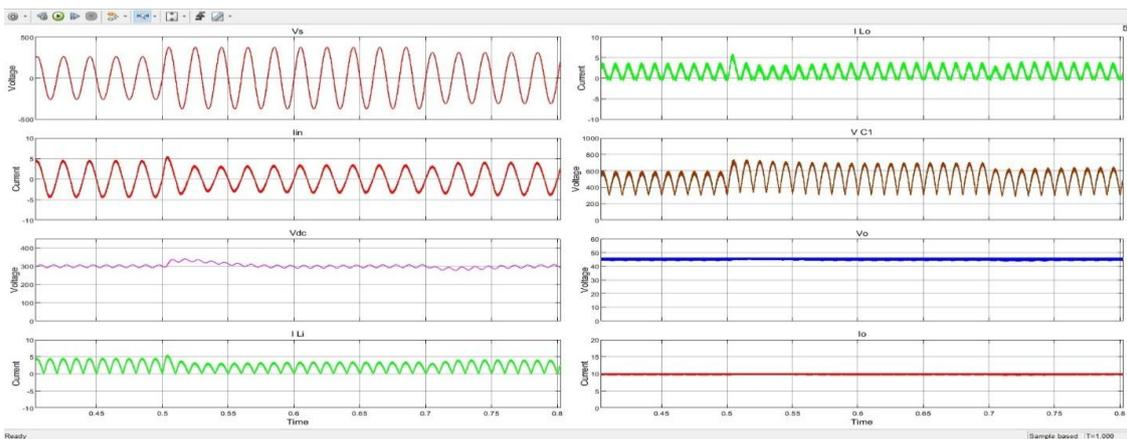
**Fig. 17:** Performance of CUK+PSFB at RL Load
