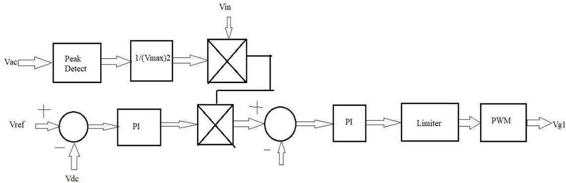
**Fig. 7:** control of CUK converter
