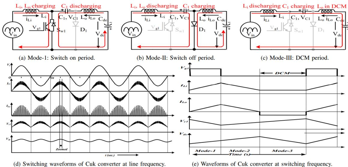
Fig. 3: Modes of Operation of CUK converter in DCM
